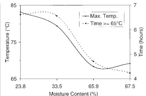
Figure 6. Comparisons are made between percentages of moisture content, the maximum temperature attained and the duration in hours at or above 65°C. All pile depths are equal (8 cm). Temperature readings are taken from the middle of the compost pile.
